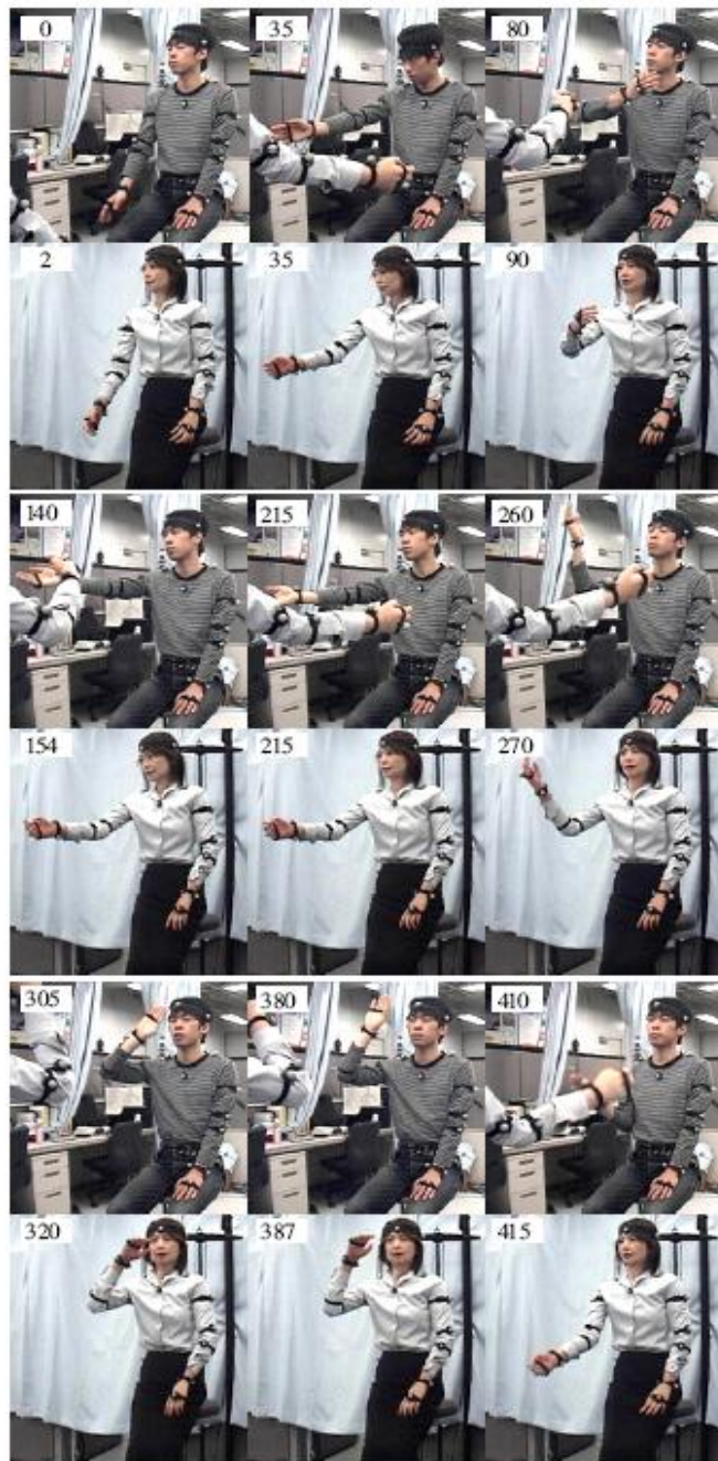
Fig. 11. The generated android's motion compared to the performer's motion. The number represents the step.
