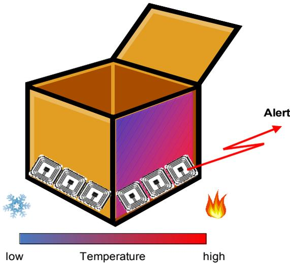
Fig. 2. Multi-tagging: example of one smart label that reports a high temperature spot, which was not discovered by other smart labels.
