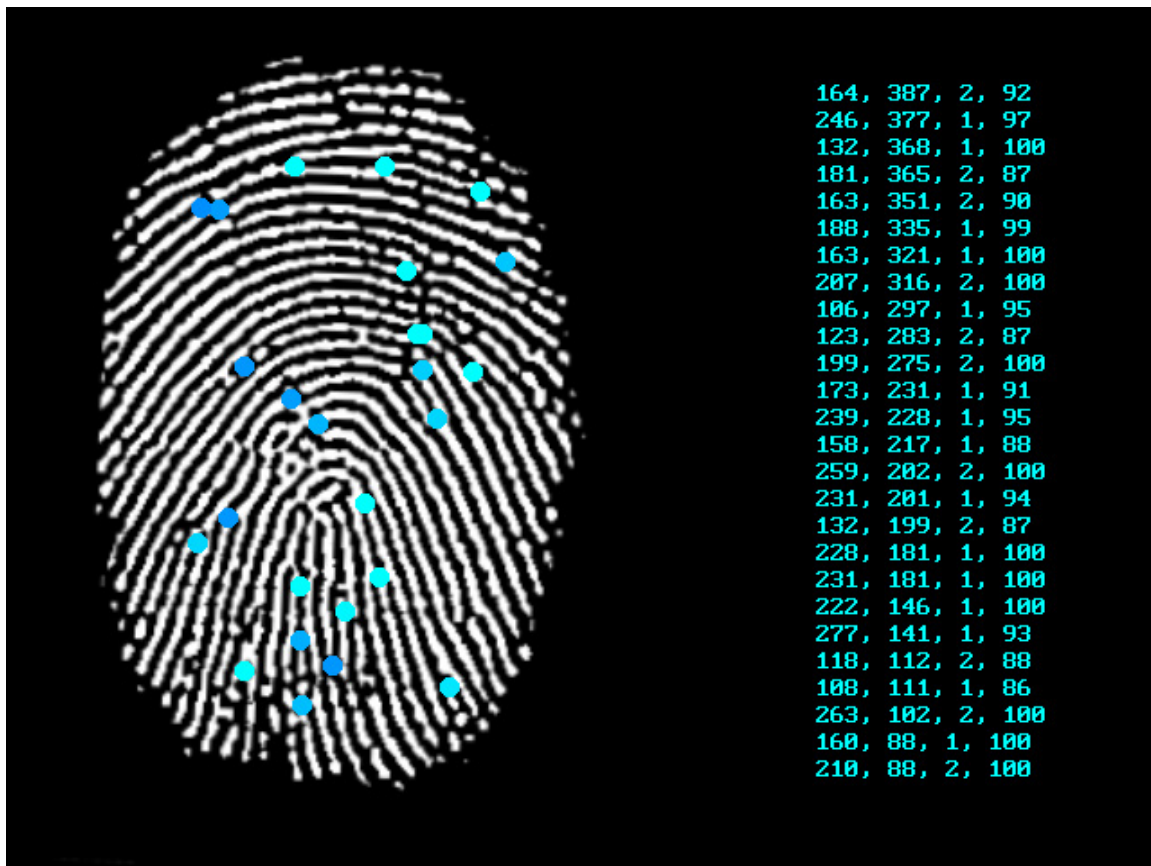
Fig 2. The Keeper shows characteristic points together with their coordinates, type code (ridge or ending) and color-coded likelihood. The Keeper also prints this information on a card, a probabilistic Icard for your reference. Keep this pint-out with your documents. It will allow you to question other non-transparent biometric readers.
